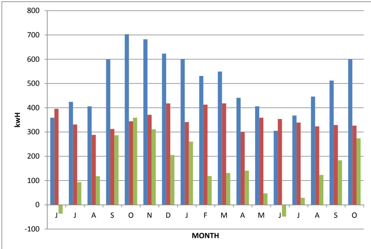
Chart showing monthly data for electricity generated (blue bars), consumed (brown bars) and exported to (or imported from) grid (green bars), over 17 months, for an all-electric house in Brisbane with 5 kWh PV unit oriented E (2.5 kWh) and W (2.5 kWh) at 23°, and assuming 20 kWh of battery storage. Electricity generated is actual data while flow to and from grid is obtained from total monthly generated minus total monthly consumed
